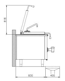
Cold Water inlet 1 (cleaning) CWII Electrical inlet (power)
